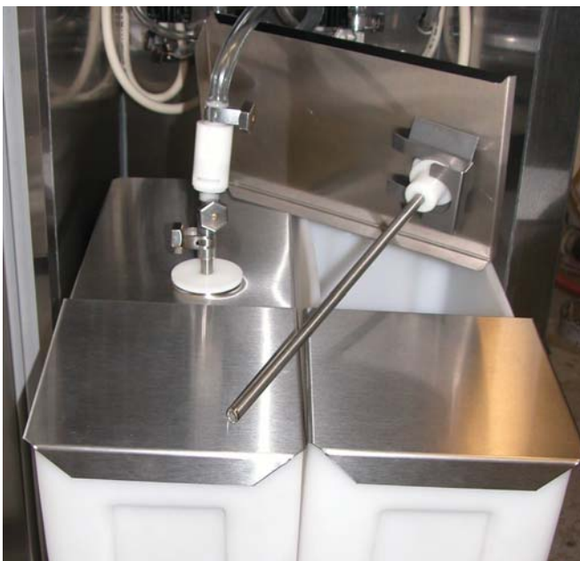
Figure 2-5 Connecting Mix Pick-up Assembly
