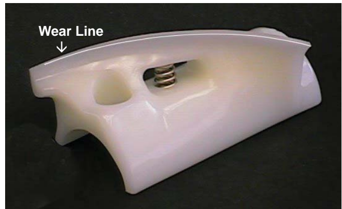
Figure 3-3 Auger Flight Wear
